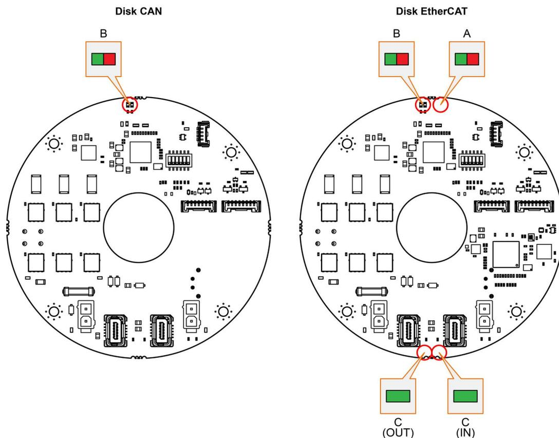
Figure 3-40 LEDs – Location
