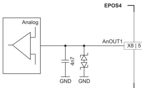
Figure 3-33 AnOUT1 circuit (analogously valid for X8a)
