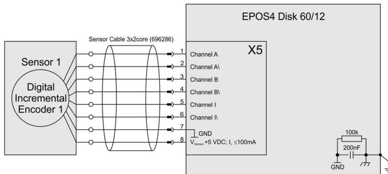
Figure 4-49 Digital incremental encoder (Sensor 1) on X5
