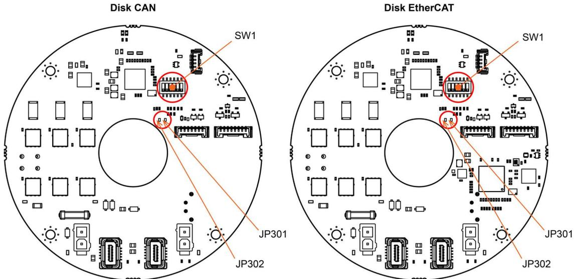
Figure 3-39 DIP switch SW1 and solder pads – Location
