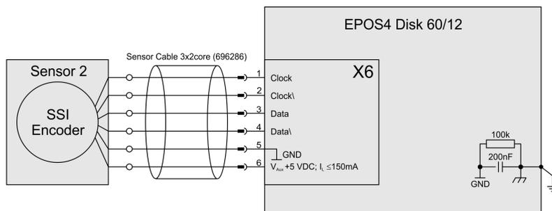
Figure 4-50 SSI encoder (Sensor 2) on X6
