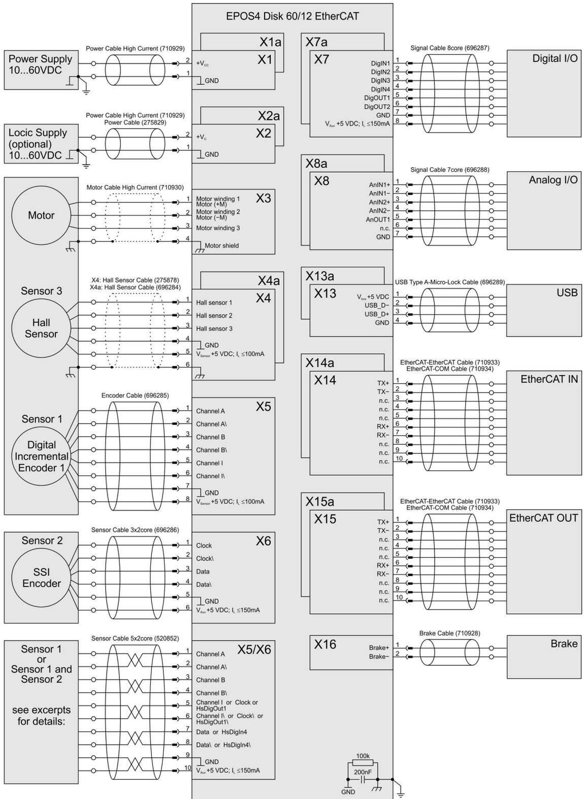
Figure 4-44 EPOS4 Disk 60/12 EtherCAT – Main wiring diagram
