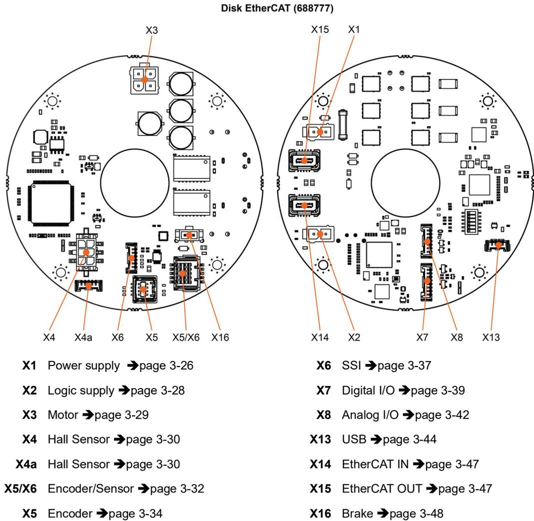
Figure 3-10 EPOS4 Disk 60/12 EtherCAT (688777) – Connectors
