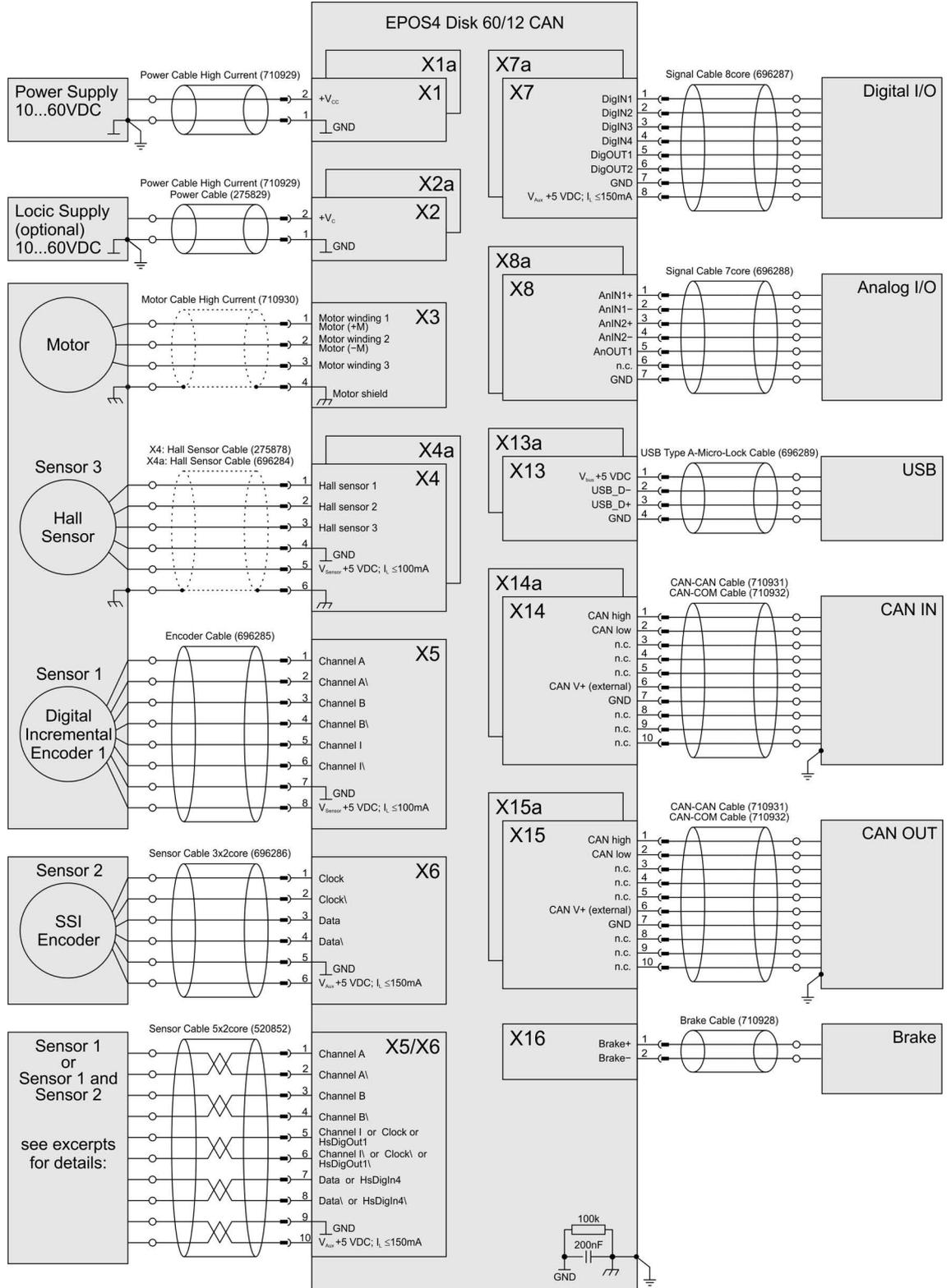
Figure 4-43 EPOS4 Disk 60/12 CAN – Main wiring diagram
