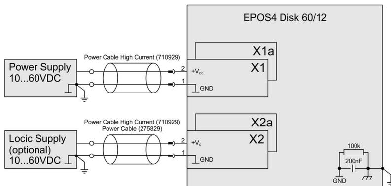
Figure 4-45 Power & logic supply
