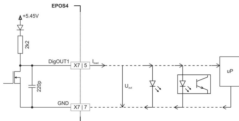
Figure 3-30 DigOUT1 “source” (analogously valid for DigOUT2 and X7a)
