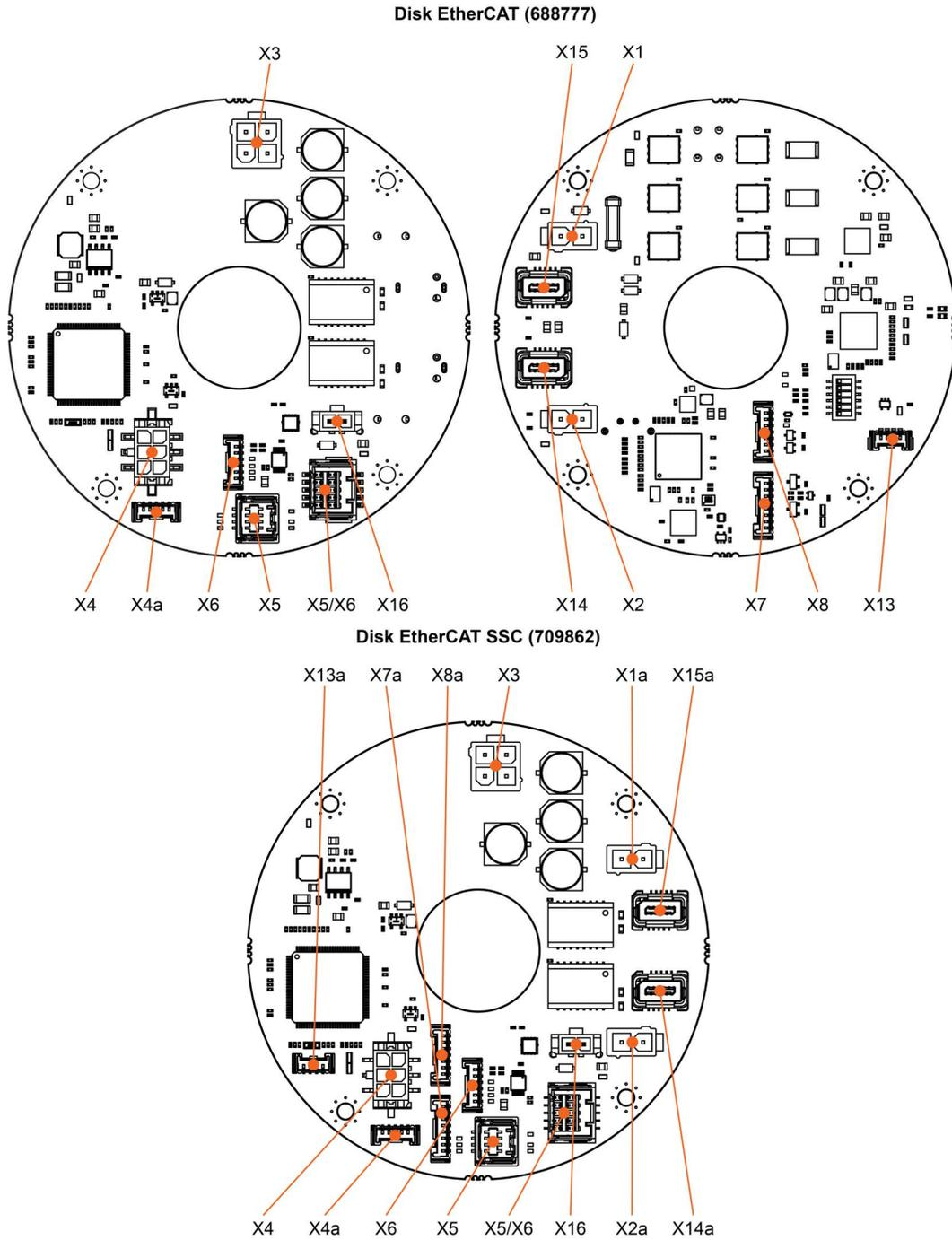
Figure 4-42 Interfaces – Designations and locations on Disk EtherCAT
