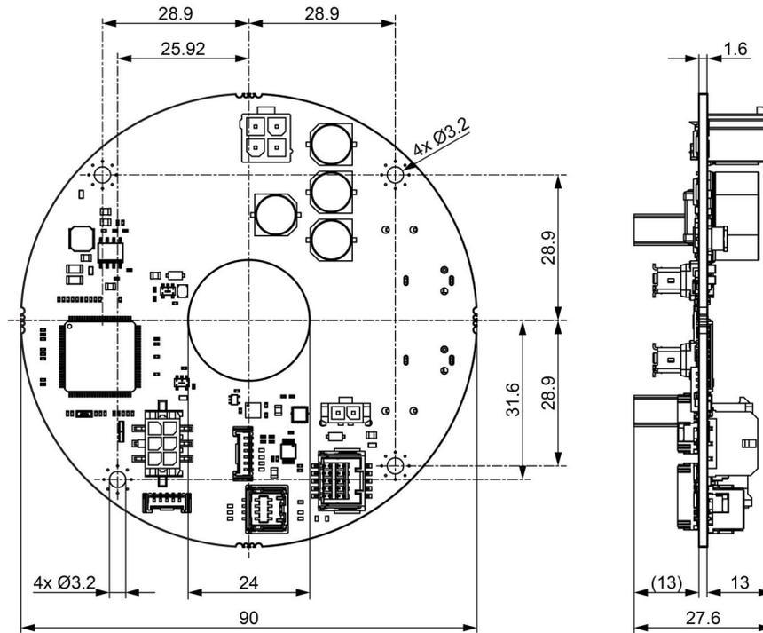
Figure 2-4 EPOS4 Disk 60/12 CAN (688775) – Dimensional drawing [mm]
