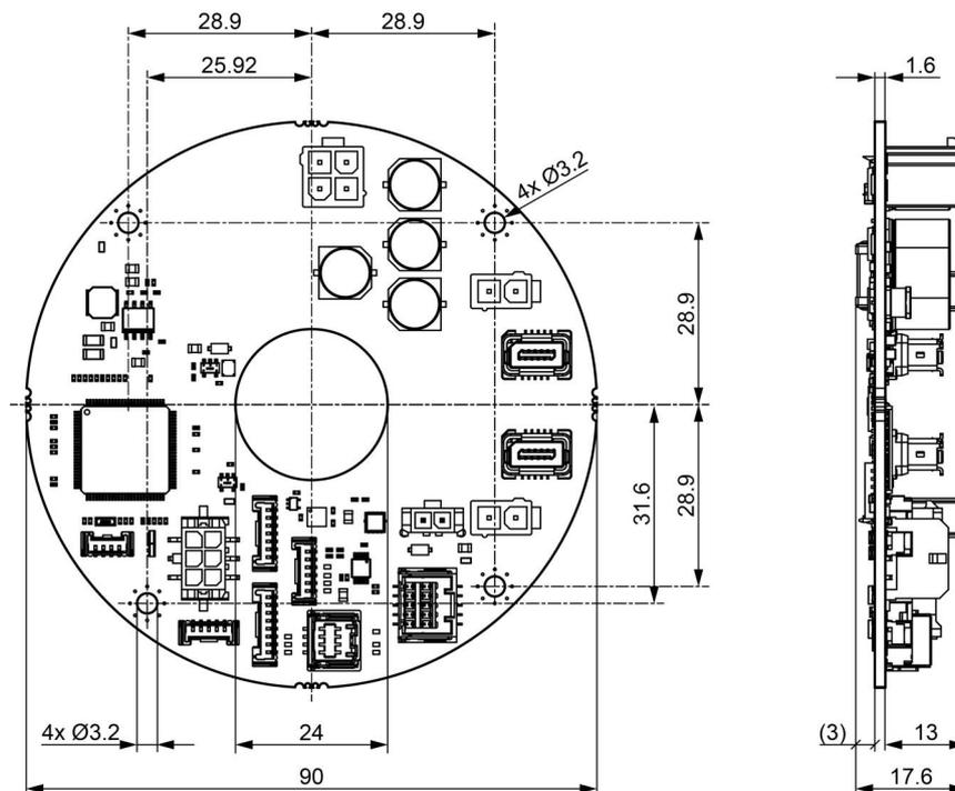
Figure 2-5 EPOS4 Disk 60/12 CAN SSC (709859) – Dimensional drawing [mm]
