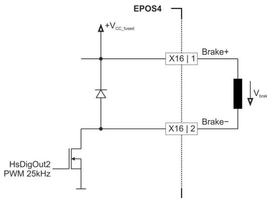
Figure 3-38 HsDigOut 2 (Holding Brake only) circuit
