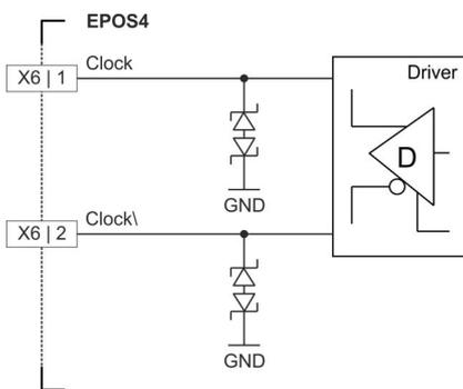
Figure 3-25 SSI absolute encoder clock output (analogously valid for HsDigOut1 and X5/X6)
